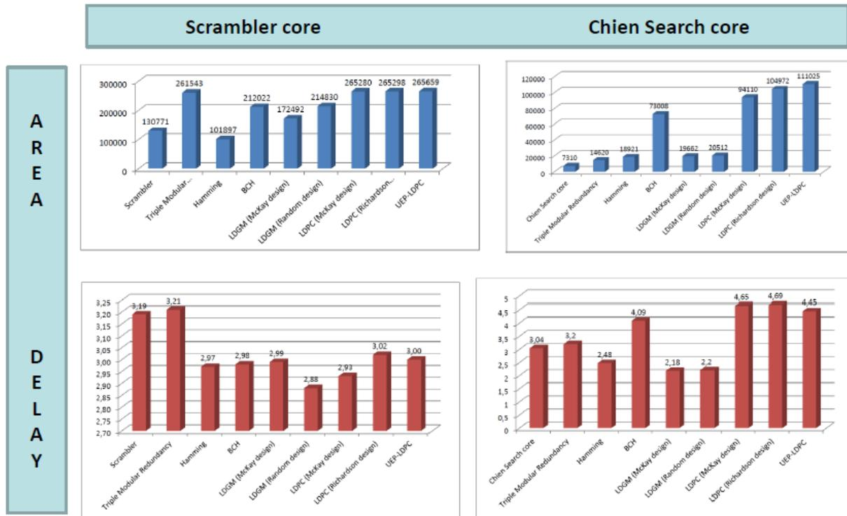
Figure 2-13: Area & timing Analysis on IP cores using CPE methodology.
