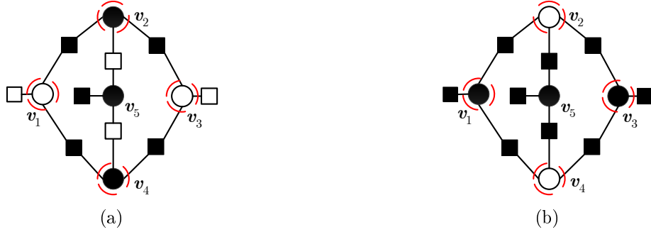
Figure 4.1: a) A three-bit pattern, b) the pattern in the second iteration of GDBF.
