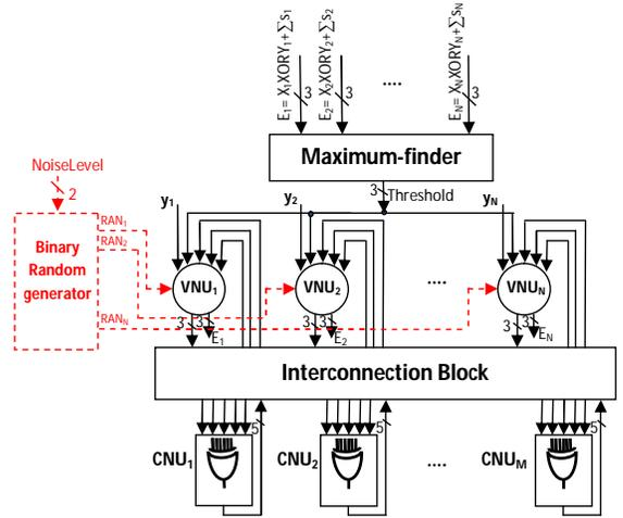
Fig. 3. Global architecture of PGDBF compared to the original GDBF
