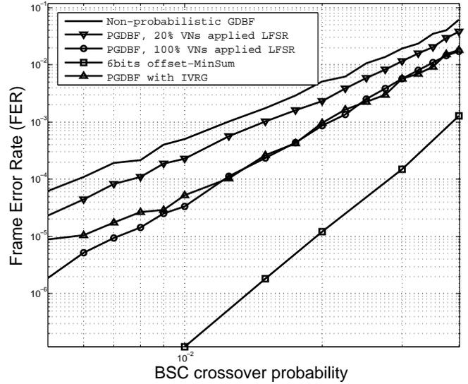
Fig. 4. FER performance comparison of the different decoders on the (N=155, K=64) Tanner code
