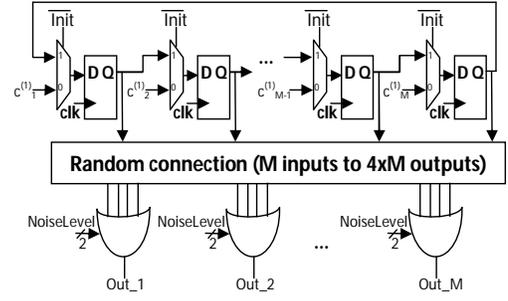
Fig. 2. Architecture of Intrinsic-valued Random Generator
